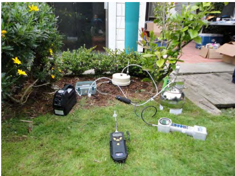
Apparatus used to sample soil gas near a building.
