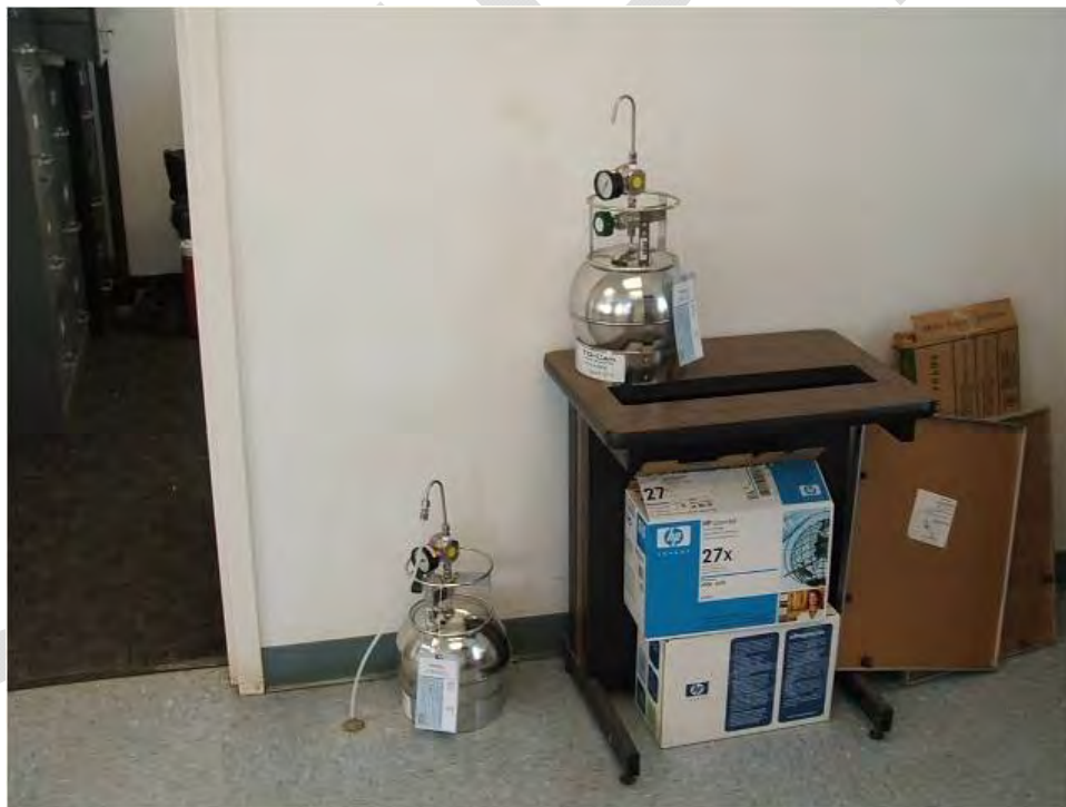
Summa canisters are used to collect a subslab sample (lower left) and a companion indoor air sample (center) in an office building.
